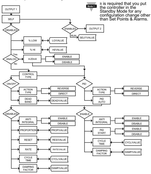
Figure 3.9 Flow Chart for Output 1
